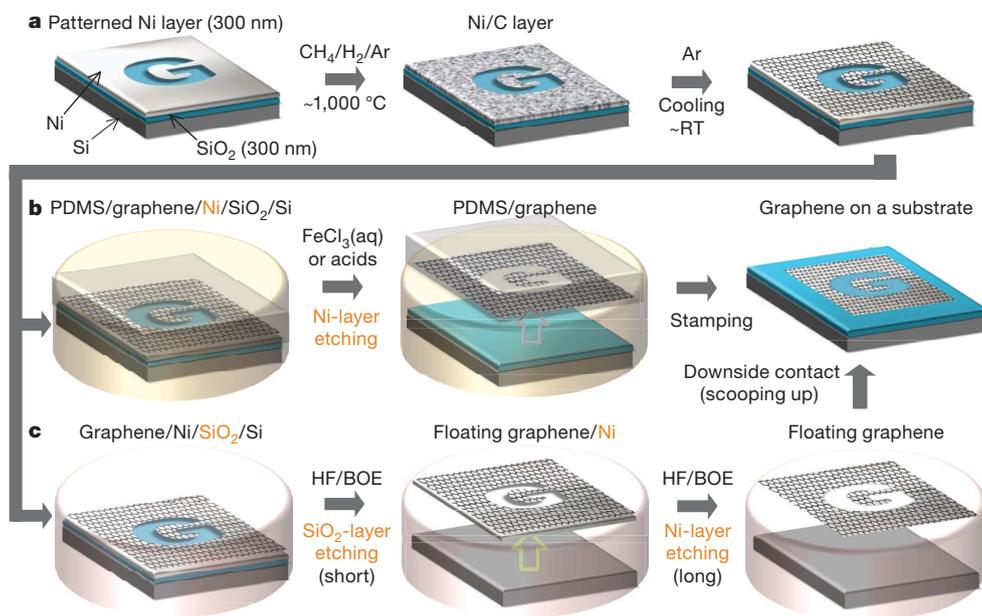
**Figure 1 | Synthesis, etching and transfer processes for the large-scale and patterned graphene films.** **a**, Synthesis of patterned graphene films on thin nickel layers. **b**, Etching using FeCl<sub>3</sub> (or acids) and transfer of graphene films using a PDMS stamp. **c**, Etching using BOE or hydrogen fluoride (HF) solution and transfer of graphene films. RT, room temperature (~25 °C).
