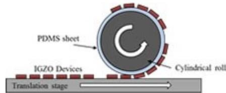
Illustration of the load-controlled roll transfer process of thin-film transistors to a PDMS substrate. Image credit: Dr. Jae-Hyun Kim and Mr. Bongkyun Jang of the Korea Institute of Machinery & Materials. Click image to enlarge.
