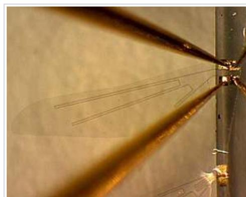
Photograph of a graphene–organic dragonfly wing microactuator
