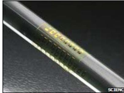
The neutral mechanical plane is the layer in a material where there is zero strain. The silicon circuits can be wrapped around curved surfaces
