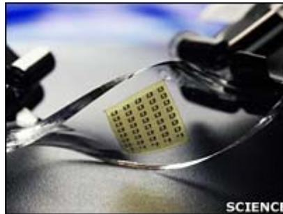
The stretchy circuits could be used in wearable health monitors
