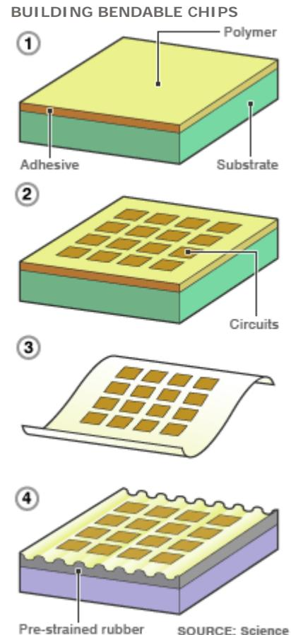
1. Plastic sheet is bonded to a rigid substrate with adhesive
